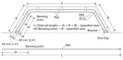
1. At the rail bending point, align the 0° point of the bender with the end of the clamp and secure.
